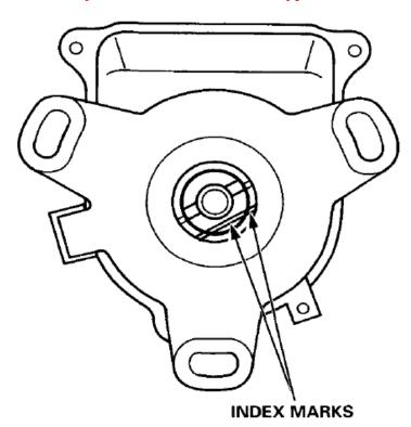
\* Align the index mark on the distributor housing with the index mark on the end of the shaft
