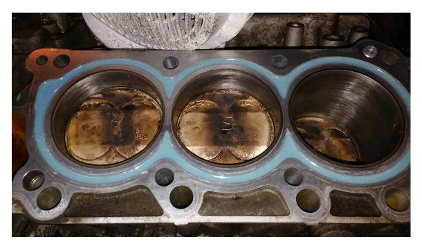
9. when epoxy is fully cured place head gasket over the block serface then mark water ports in the gasket to the block with a marker.
