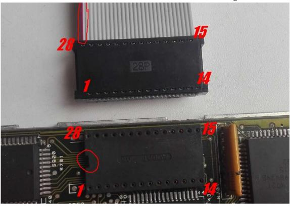
It is necessary to navigate the red or white strip on the cable and the cutout on the socket, which should be on one side!
