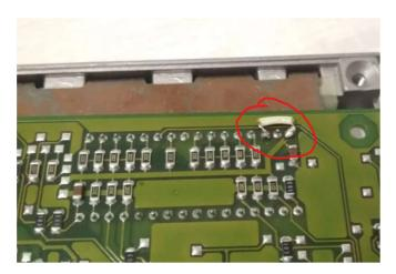
After all the manipulations, with the correct connection, after turning on the ECU (ignition) on the MotronicRT board, the "Status" indicator should light up.
