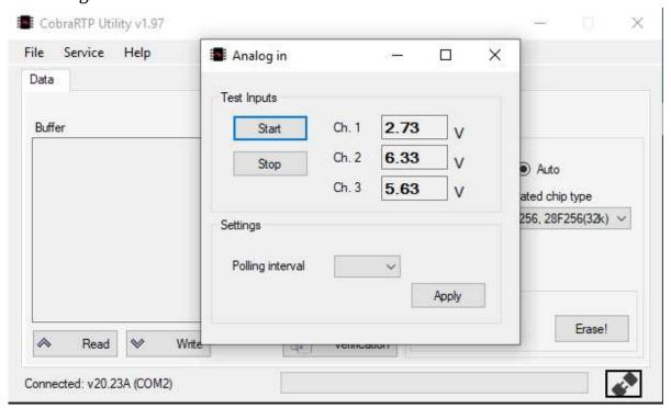
After that, the current voltage of each channel in real time should be displayed in the output windows of the corresponding channel.
