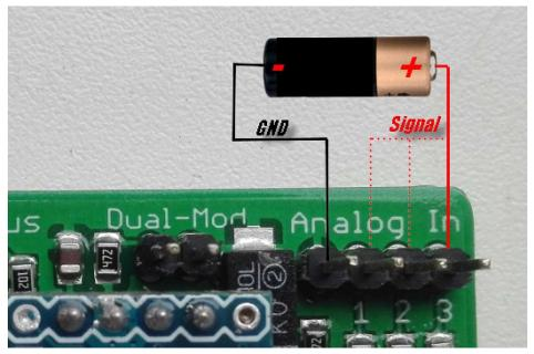
The signal conductor (in this case +) can also be connected simultaneously to all 3 channels.
