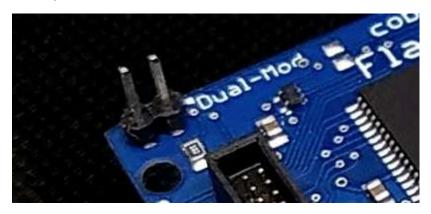
Dual-mod works only in emulation mode 28F200, 28F400, 29F200, 29F400, i.e. with firmware 256-512kB, tk. FlashOnline total memory 1024kB (100000h) or 2 conventional blocks of 512kB each. **When emulating 29F800, this function does not work.!**
