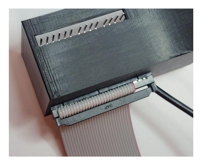
Another tip would be to push towards the analog pin side, with the pins through the hole, move them up towards the top of the hole as much as you can that will get you more room on the bottom inside where the pins wont go over the plastic edge
