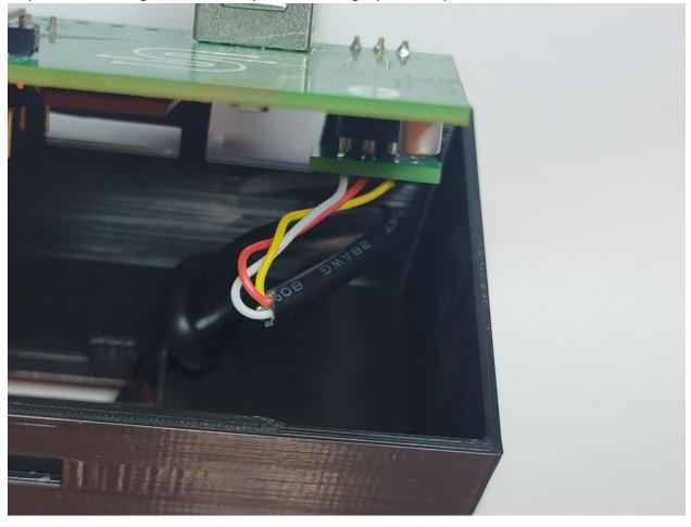
Step 2, the cn2 wire goes on with the yellow on the right pin in this position
