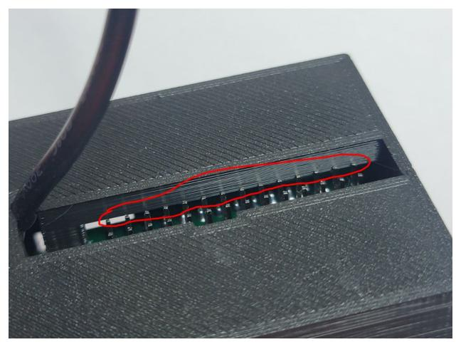
Step 6. Then when you got it in and like this, the cables ready to go on. The cable takes a little alignment as well you gotta align the tab with the cutout on the case, then move the snake/adapter around until the pins line up with the cable.
