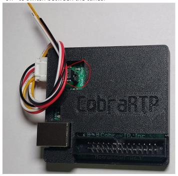
If you are not using the analog inputs, also remove the wires/pigtail and store them somewhere for possible future use.
