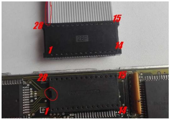
It is necessary to navigate the **red stripe** on the cable and the cutout on the socket, which should be on one side! If connected correctly, after on ignition, the "Status" LED on the MotronicRT board should light up.
