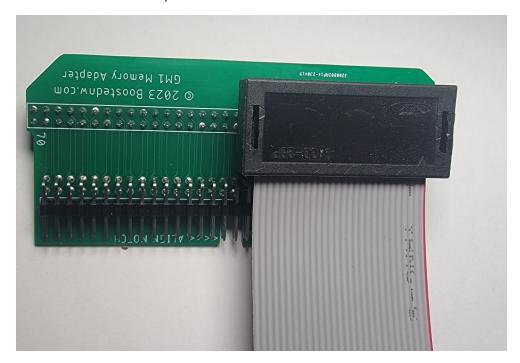
When using with a Moates Ostrich/Ostrich2 Unit & cable, the cable should be plugged into the adapter like this(below):
