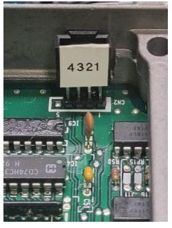
Plug the ECU side in with the latch facing outwards towards the case, another way to tell is verify the black wire in the connector is going to PIN #1 Always or you could damage your Datalogger.
